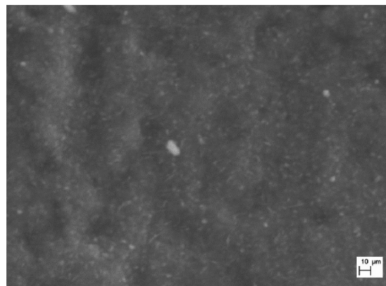
Fig. 1. SEM photograph of SiO 2 fresh films doped with 0.28% Nd 2 O 3 .
