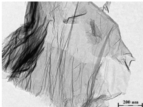
Fig. 1. TEM micrograph of 1 mg/mL rGO dispersion in ethanol.
