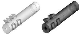
Fig. 2. Model building and meshing
