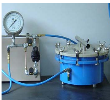
Fig. 1. Pressure plate test device
