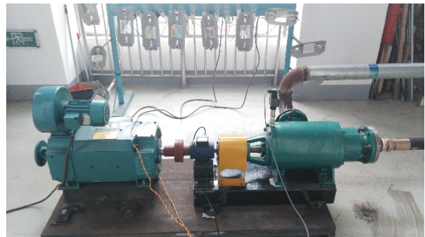
Fig. 7. Shaft power load and dissipation module
