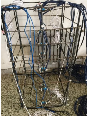
Fig. 1. Layout of temperature measuring points
