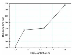
**Fig. 5.** Relation between H63L content and thickening time.
