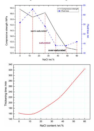
**Fig. 3.** Upper: relation between content of NaCl and compressive strength and fluid loss; lower: curve of content of LATEX *vs.* thickening time
