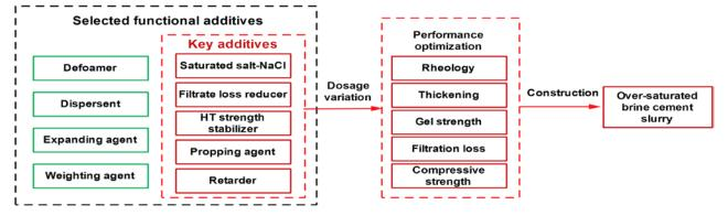
Fig. 1. Experimental design of constructing over-saturated brine cement slurry.
