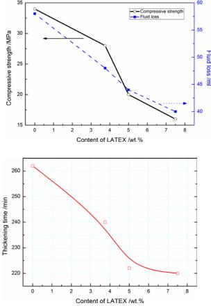
**Fig. 2.** upper: relation between content of LATEX and compressive strength and fluid loss; lower: curve of content of LATEX *vs.* thickening time.
