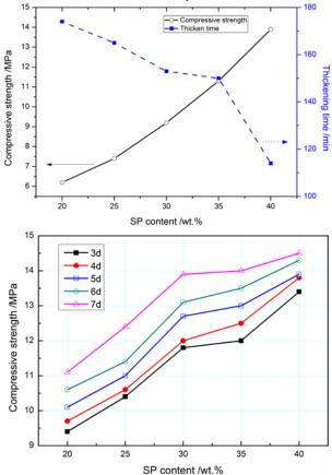
**Fig. 4.** Upper: relation between SP content and compressive strength and thickening time; lower: relation of SP content and compressive strength after a long-term high temperature.
