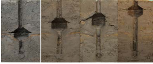
Fig. 8 Failure behavior after the pile being taken
