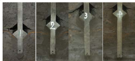
Fig. 7. Failure behavior of the soil for different model piles
