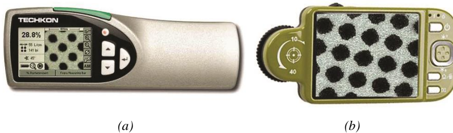
Figure 2. Measuring devices: a) Techkon spectroplate; b) Vitiny VT-300 digital microscope.
