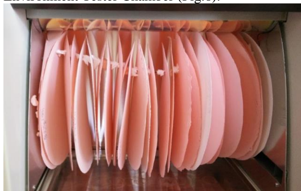
Fig. 6 Paper samples in the Suntest apparatus
