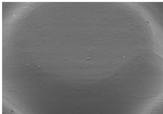
Fig.3. Microphotography of dots on plates made in a) oxygen environment, b) in an inert atmosphere.
