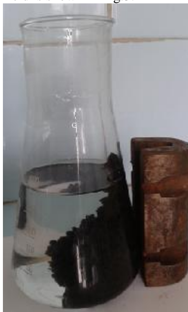
Fig. 3. Magnetic separation of magnetic polyurethane foam particles under an external constant magnetic field
