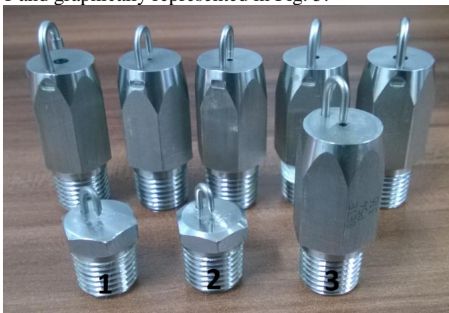
Fig. 3. Three of the tested BETE nozzles ( http://www.bete.com/pdfs/BETE_PJ.pdf ): PJ6 with orifice diameter of 0.152 mm (1); PJ10 with orifice diameter of 0.254 mm (2), P54 with orifice diameter of 1.37 mm (3).
