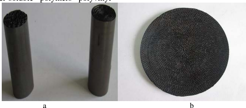
Fig.1. The metal blocks for the laboratory samples of catalysts: a - perspective view; b - cross-sectional view
