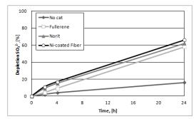
**Fig. 4.** Depletion of  $SO_3^{2-}$  using three different catalyst
