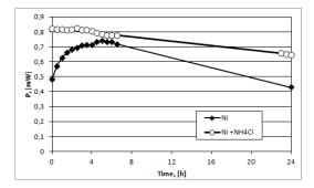
Fig. 5. Power in time using nickel-plated graphite fiber
