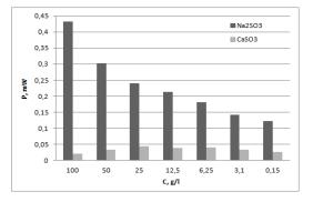
**Fig. 3**. Influence of the concentration of Na<sub>2</sub>SO<sub>3</sub> and CaSO<sub>3</sub> on obtained electrical power
