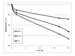
**Fig. 8**. Depletion of  $SO_3^{2-}$  using three different oxidizers
