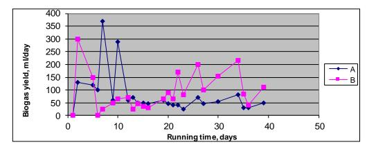
Fig. 1. Daily biogas yield. Samples A1 and B1
