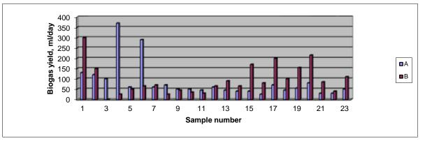
Fig. 2. Biogas yield for longer period of time (experiment 1).
