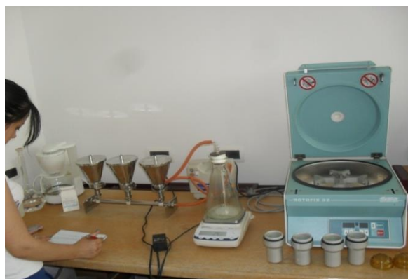
Fig. 1. Pilot scale apparatus and centrifuge used for beer filterability monitoring in experimental scale.
