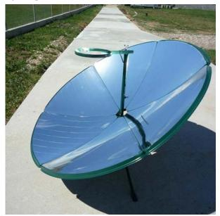
Fig. 1. Solar parabolic cooker.
