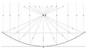
Fig. 2. Principle of action of the solar parabolic cooker (mirror): AB – diameter of the reflector; OF – focal distance.
