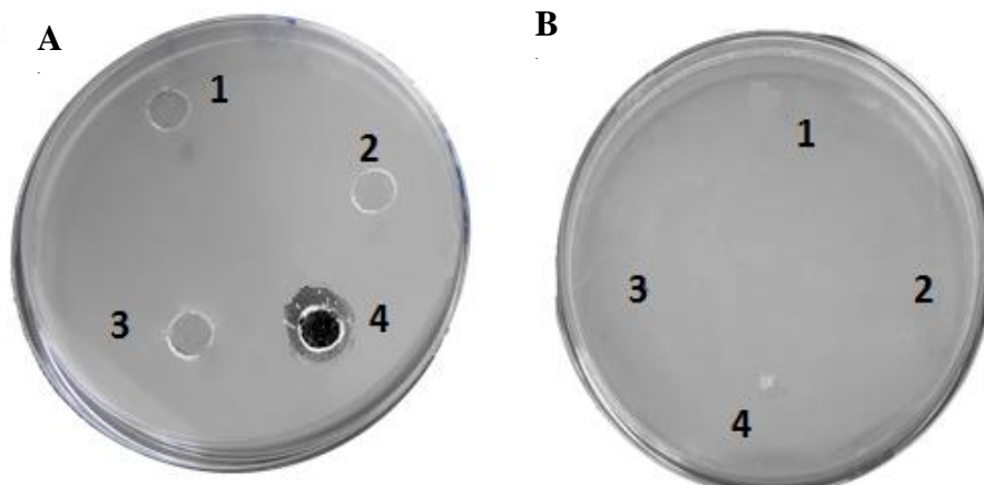
Fig. 1. A) Antimicrobial assays against Gram-negative E.coli of isolated fractions: A (spot 1), B (spots 2) and C (spots 3). Antimicrobial assays via agar well diffusion method against Gram-negative E.coli of isolated Fraction 1 (spot 4). Each fraction was applied on the agar medium in 50 \mu l of the peptide solution. B) No activity is shown in any of the fractions after dilutions (1/2, 1/4, 1/8 and 1/16) from the starting concentration.
