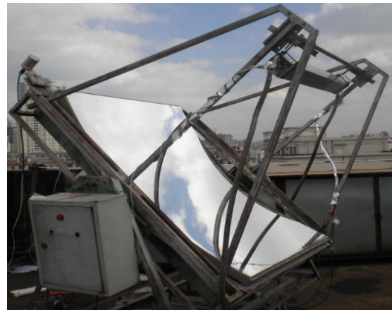
(b) Picture of Solar trough concentrating PV/T system
