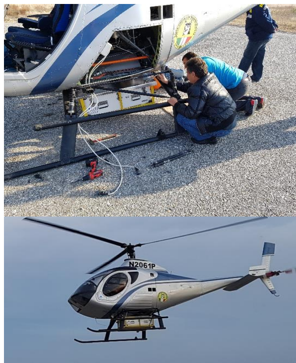
Fig. 2. The spectrometry system installed on Schweizer 333 (269D).
