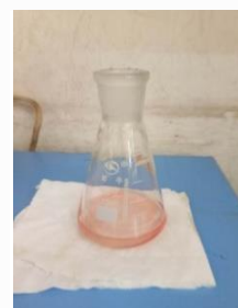
Fig.1. The color of titration endpoint for acid - base titration
