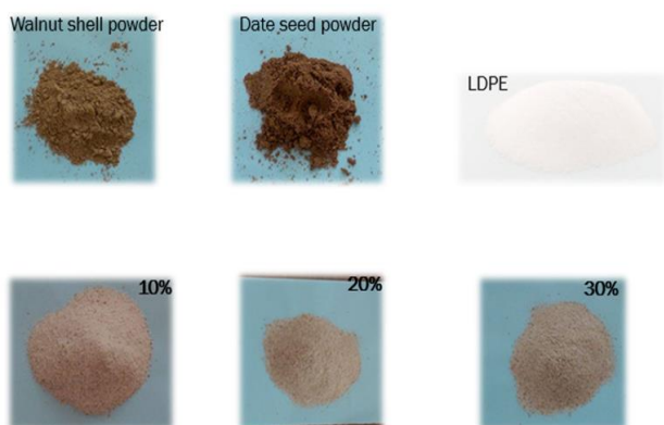
Fig 2. Composite preparation with different proportions
