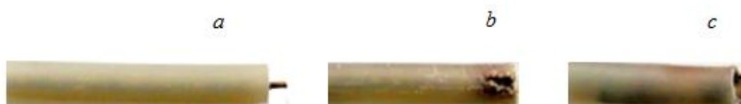
Fig. 1. Cable-electrode and characteristic failures during its operation (a) before treatment, (b) at W = 600 J, and (c) at W = 1350 J.
