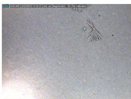
Fig.4. Microscopic image of the perovskite coating at the optimized deposition of perovskite ink on the glass/ITO/ZnO:Ga 2 O 3 substrate
