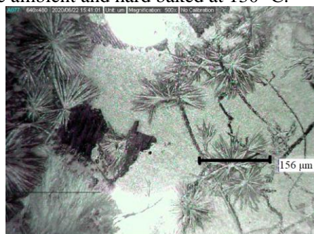
Fig.2. Microscopic image of the perovskite coating at the initial deposition of perovskite ink on the glass/ITO/ZnO:Ga 2 O 3 substrates
