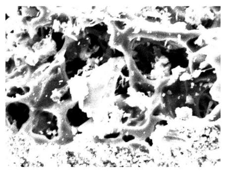
Figure 1. Photomicrograph of activated carbon obtained from rice husk
