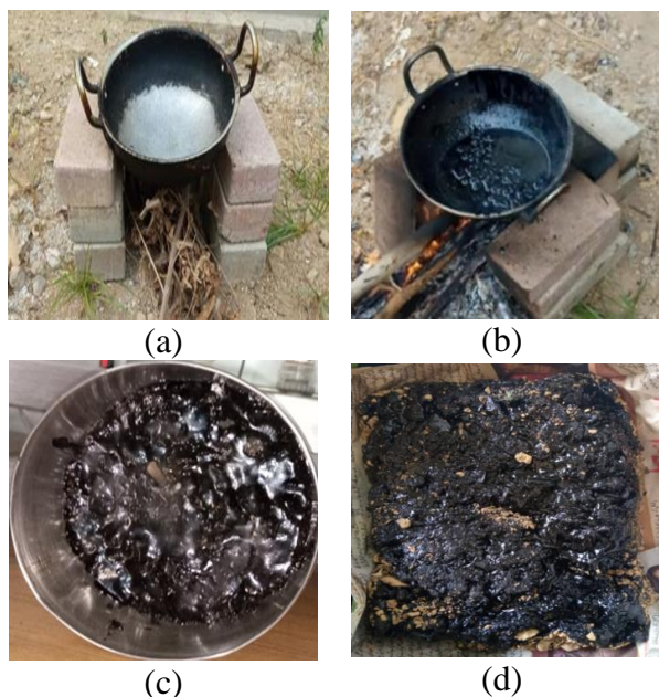
Fig. 6. (a) Open flame setup; (b) PCA and bitumen mix in the process; (c) Product of open flame process (d) Block of PCA-bitumen mix prepared in the newly designed equipment
