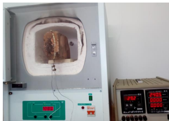
Fig.5. Approbation of the method for determining the thermal state of the lining on a physical model in laboratory conditions
