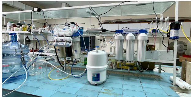
Fig. 4. Cascade spring water purification system
