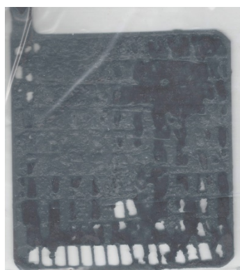
Fig. 6. Negative plate with CB additive after formation process.
