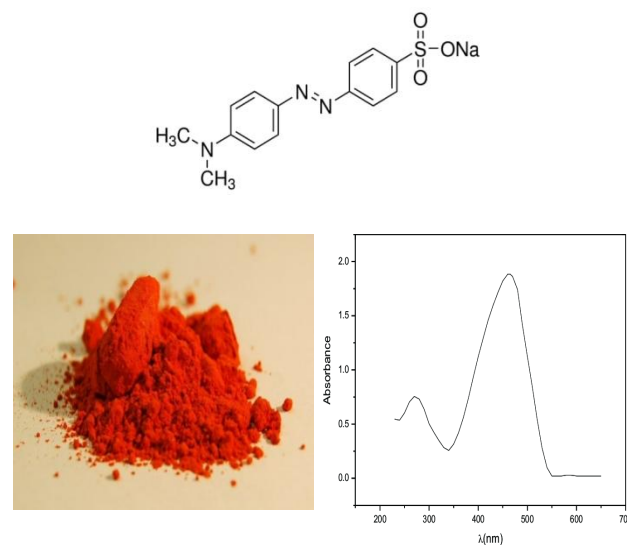
Figure 2. Structure and UV-vis spectrum of the photosensitive compound (methyl orange)
