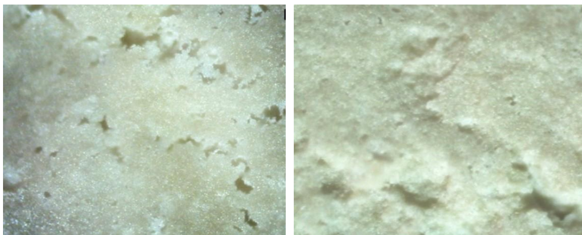
Figure 3. SEM microphotographs of barium titanate-based ceramic samples synthesized from blend D0 at 1300°C
