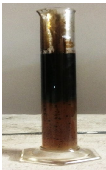
Figure 2. Bio-oil formed by microwave pyrolysis
