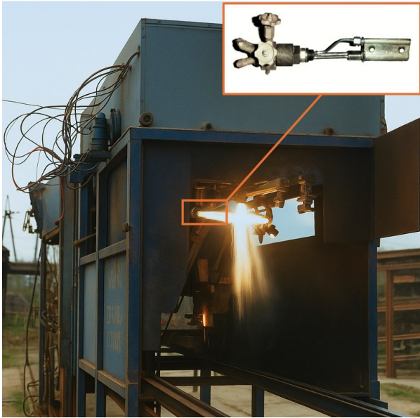
Fig. 2. Flame pit of the production line with four machine kerosene-oxygen thermal tools, operating in automatic mode, for spraying natural materials on products.
