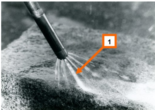
Fig.7. Position of the torch to the granite processing surface: 1 - structure of the torch.
