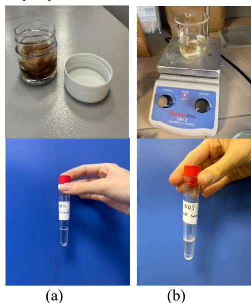
Figure 7. (a) 24 th h of dissolution of disk cotton coated with the plant extract mixture in PBS (b) 48 th h of dissolution of disk cotton coated with the plant extract mixture in PBS.
