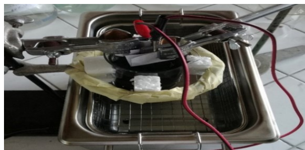
Fig. 3. Experimental setup for combined ultrasonic treatment and electrolysis.
