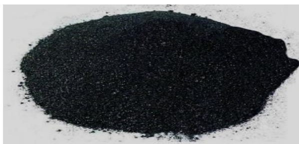
Fig. 2. Initial graphite powder
